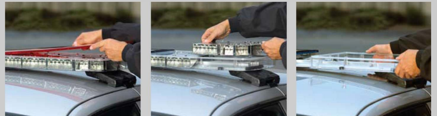
1 Remove the top dome with only four screws 2 Disconnect the ROC board. 3 The base slides off for quick replacement.
